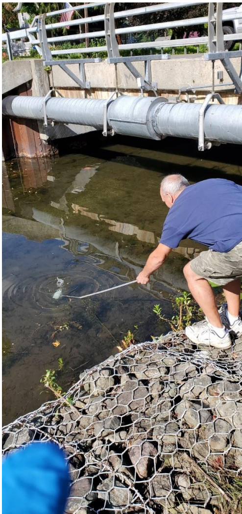
Photo 3 (above): William Boria collecting a sample from the outlet of Cassadaga Lakes using a sample pole. Photo 4 (above right): Boria collecting a sample from the Village of Mayville's well before the water is treated to remove PFAS. Photo 5 (right): Jane Conroe collecting and preparing a PFAS sample using a Cyclopure filter.
